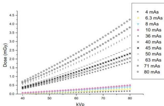
Figure 7: The graphical presentation of representative sample of dose range for tube output calculations at corresponding different mAs settings.
